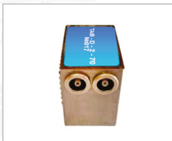
Crystal Probe: TAB-D-2-70 (70 degree, 2MHz)
