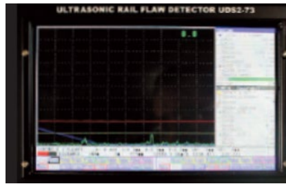
Display mode: A-Scan for one channel
