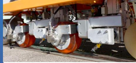
Ultrasonic electronic modules: OKOSCAN UT 73HS System employs ultrasonic single-channel modules OKO-24-UT with a frequency range of 1 to 7 MHz and PRF of up to 5 kHz.
